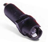
**Cloth extendable junction** When the cloth junction becomes dirty from routine testing, simply pull out 3 mm (1/8") to increase response time and stability.
